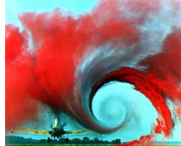
Turbulences on macroscale due to fluidic inertia
